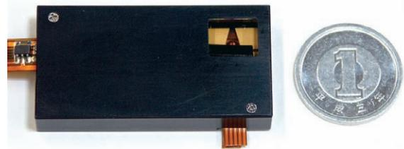
Fig.3 Prototype of ultra compact projector module
